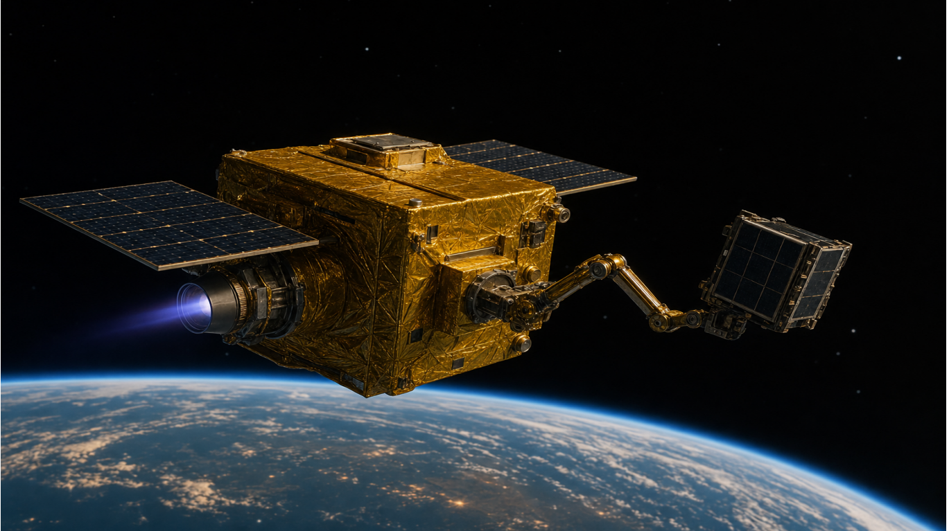
FIG. 03 SPARROW retrieval drone – gold MLI-wrapped bus, two deployable solar wings, single Hall thruster aft, 3-DOF capture arm forward holding a captured defunct cubesat. The arm grips standardized launch adapter rings on cooperative targets; net cartridge mounts on the forward face for tumbling debris.
