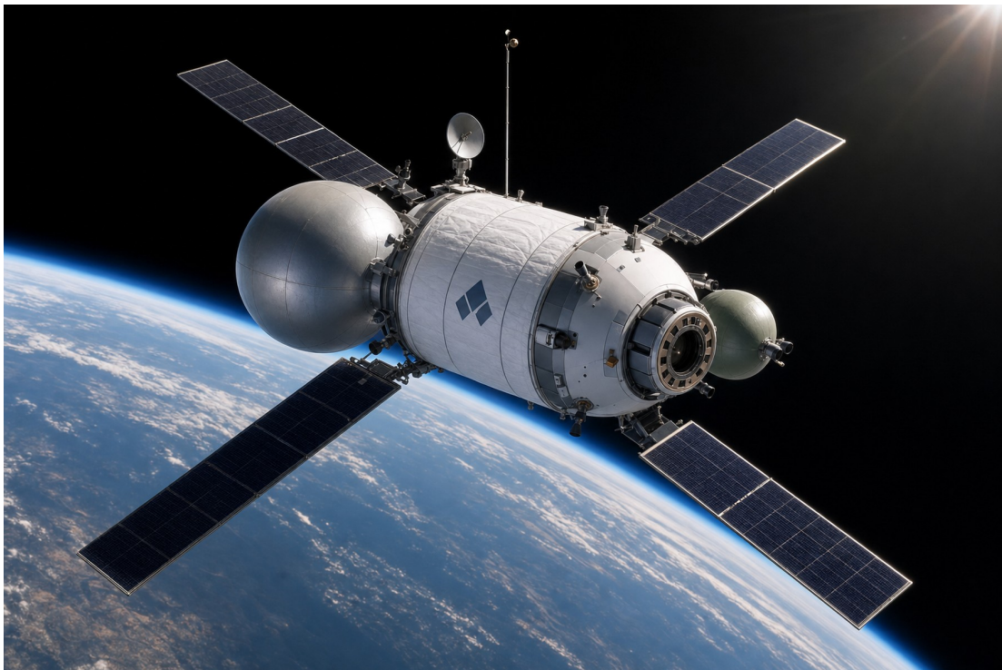
FIG. 04 Sparrow Depot — cylindrical MLI-wrapped trunk with composite-overwrapped krypton tank and diaphragm-isolated green-mono tank. Four-panel solar array, RAFTI-class docking face forward.
